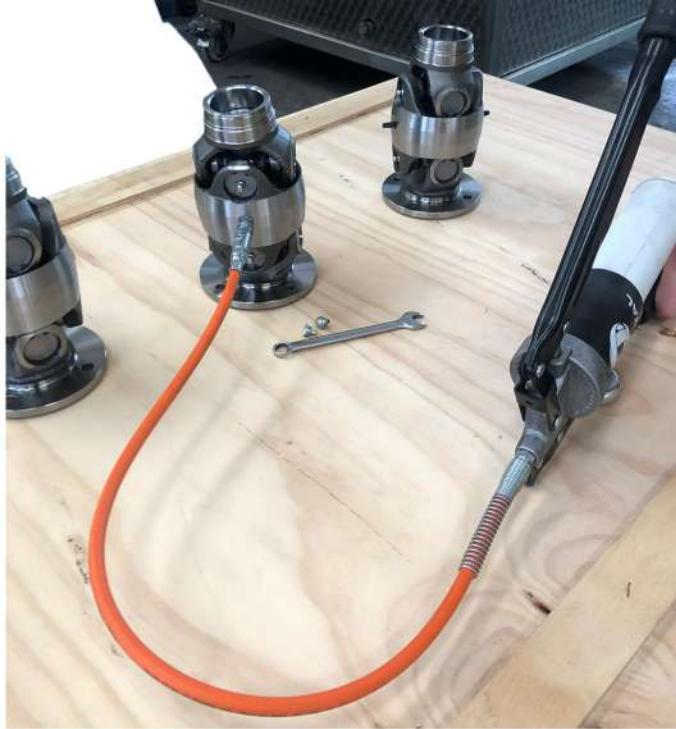
The universal joints are made by us by using on INA bearing u-joints with grease nipples to ease the maintenance.
