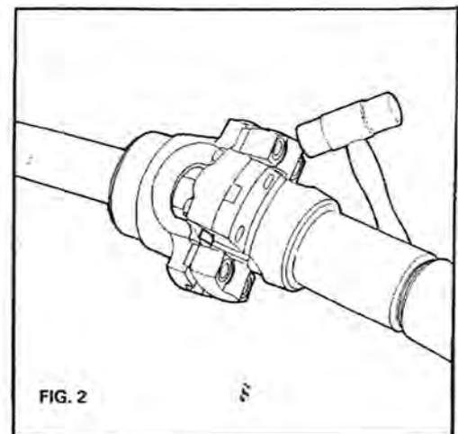
Screws must have no trace of grease or dirt at all. We do not suggest using washers, either normal or elastic.
